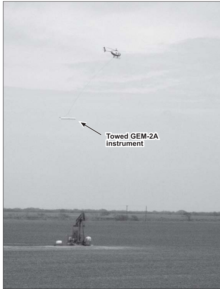
Figure 6. Hughes 369D helicopter towing the Geophex GEM-2A at survey height over the Clara Driscoll Oil Field southeast of Driscoll, Texas, February 5, 2005.
