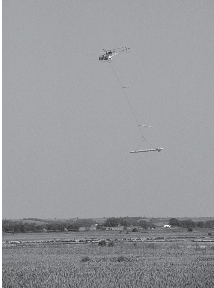
Figure 6. The DIGHEM V airborne EM system at the Montague Test Site. The lower bird contains five pairs of induction coils and is used to measure the apparent electrical conductivity of the ground. The upper bird is the Cesium magnetometer used to measure magnetic field strength.
