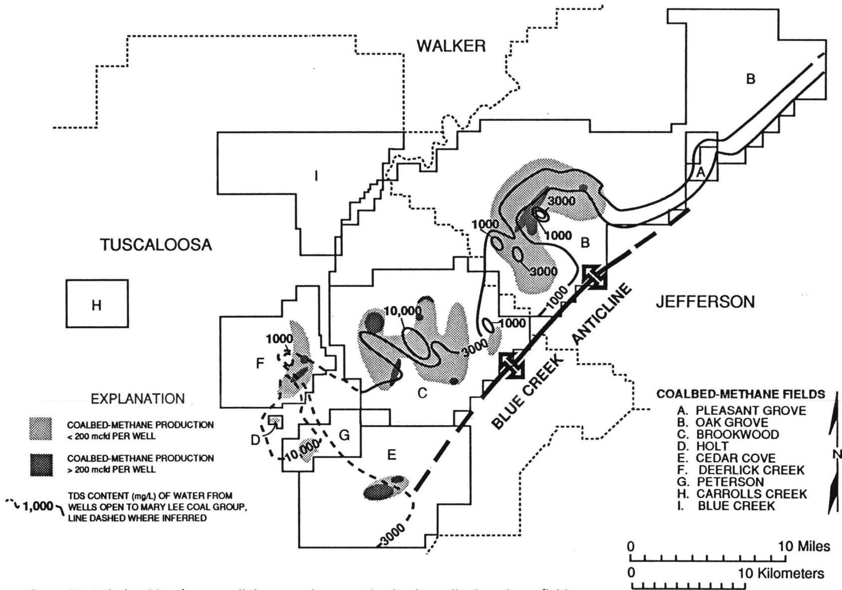
Figure 88.--Relationship of water salinity to peak gas production in coalbed-methane fields.
