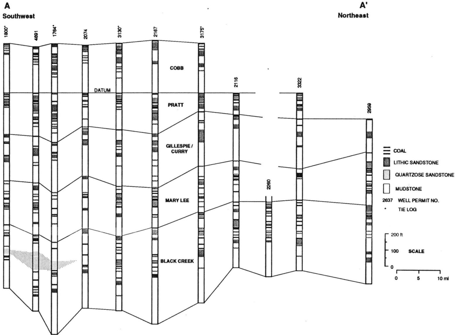
Figure 40.--Stratigraphic cross section A-A'.
