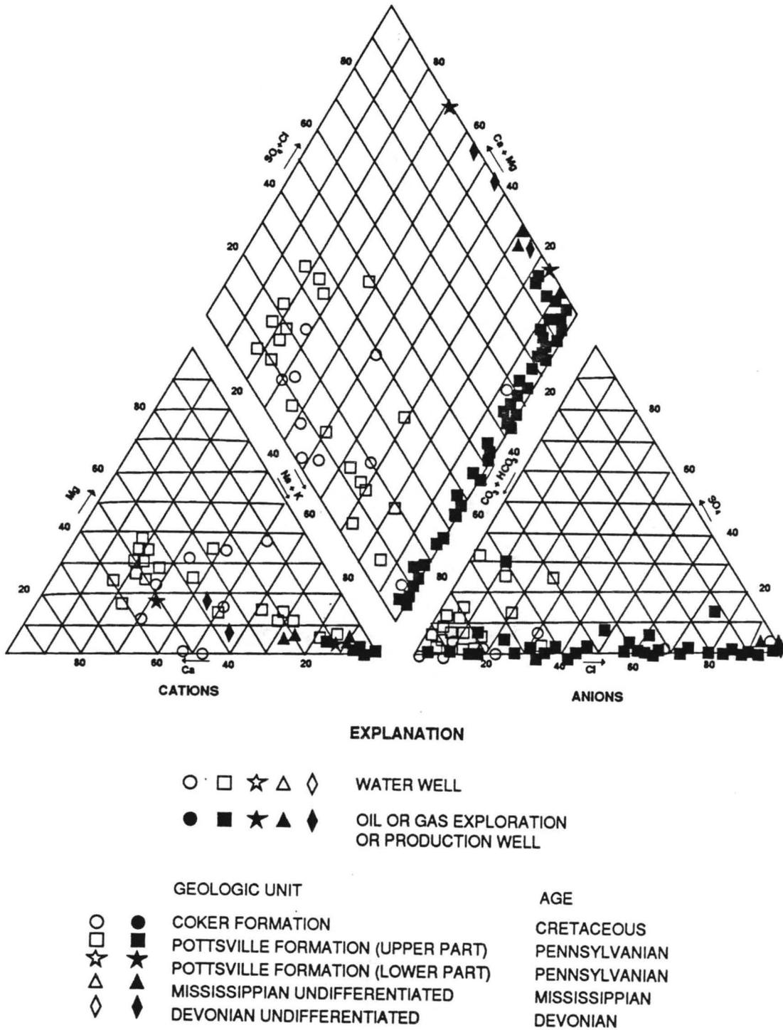
Figure 82.--Piper diagram showing stratigraphic units in relation to water type.
