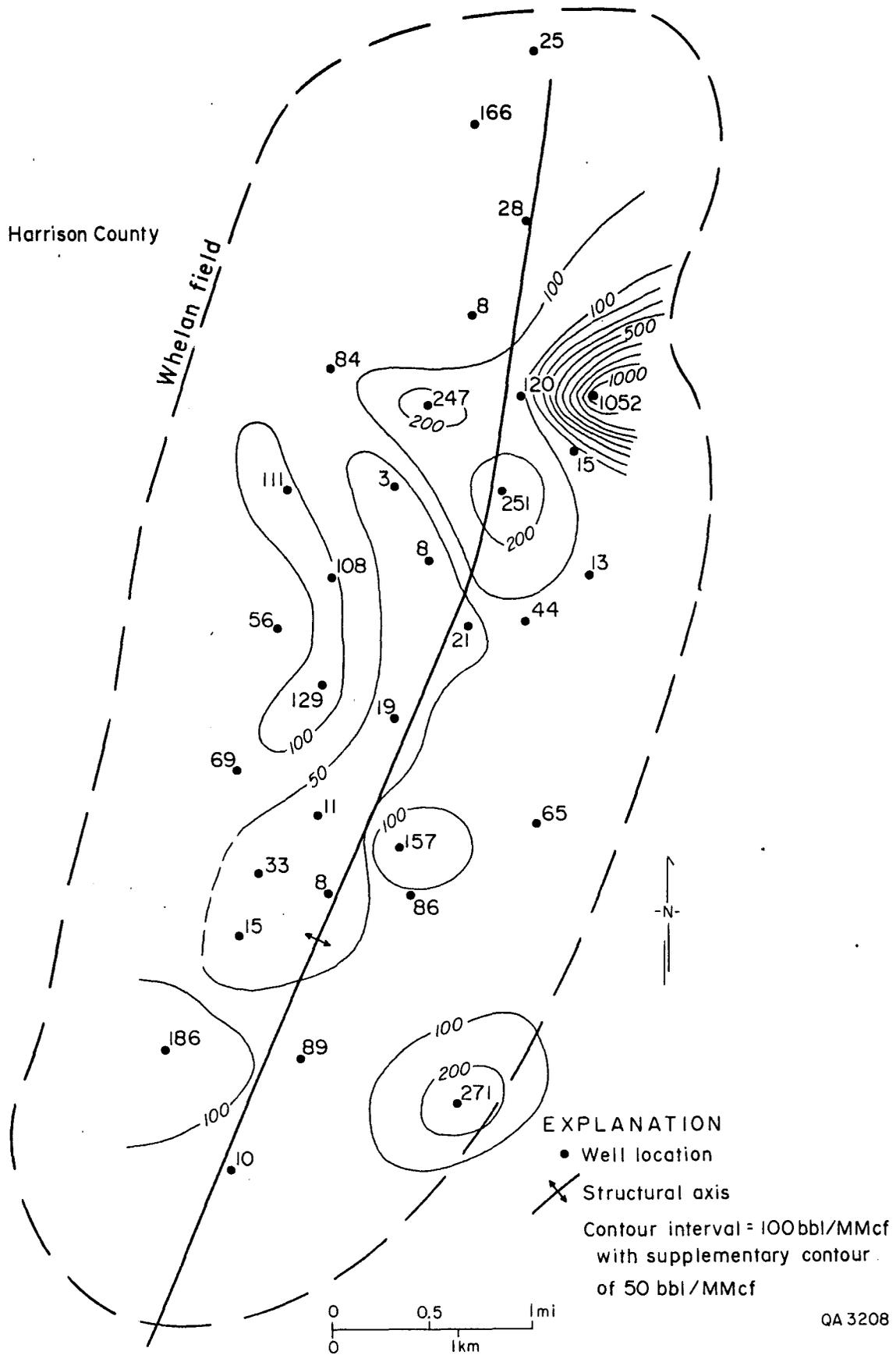
Figure 10. Distribution of initial water/gas production ratio in the Travis Peak Formation in Whelan field.
