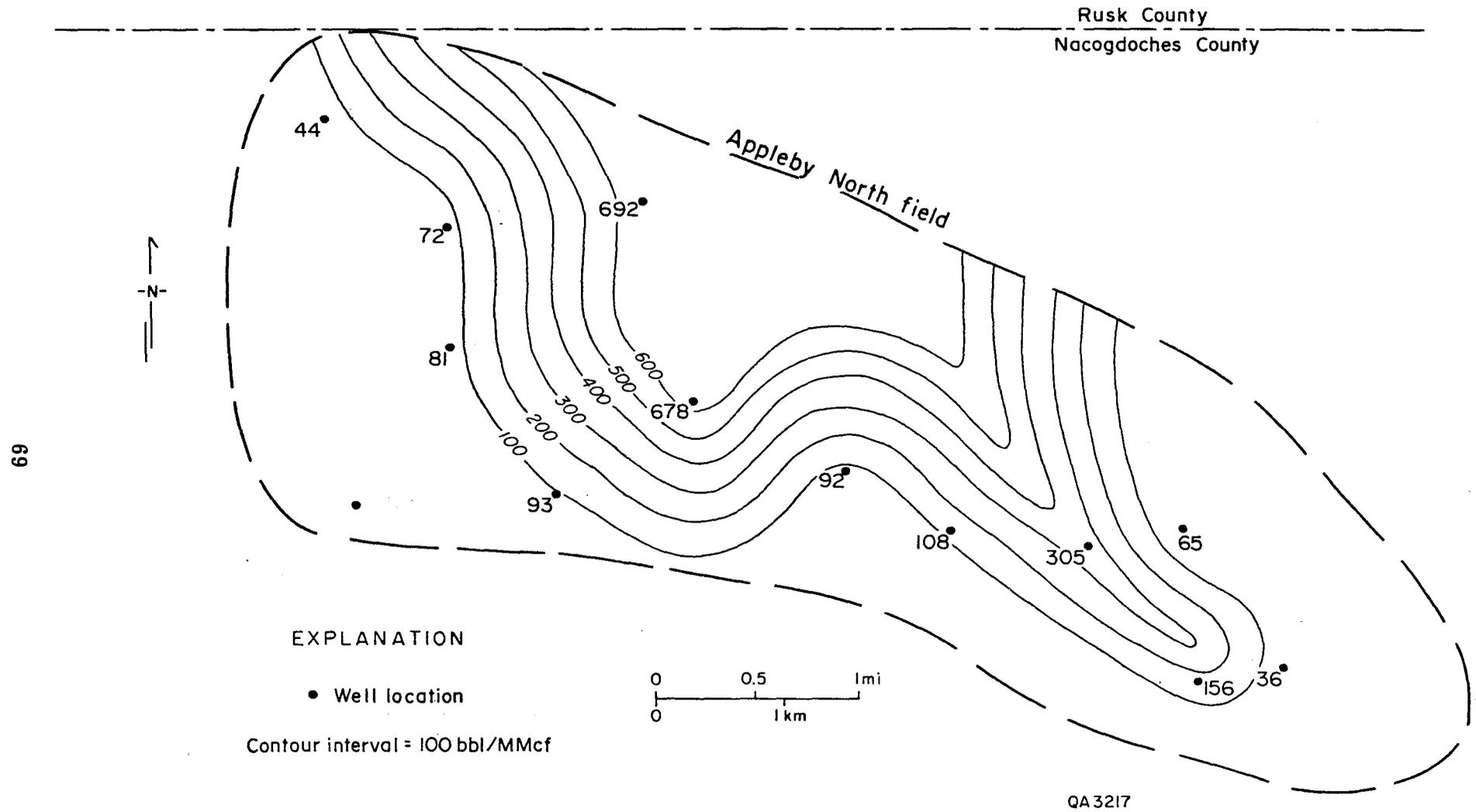
Figure 23. Distribution of initial water/gas production ratio in the Travis Peak Formation in Appleby North field.
