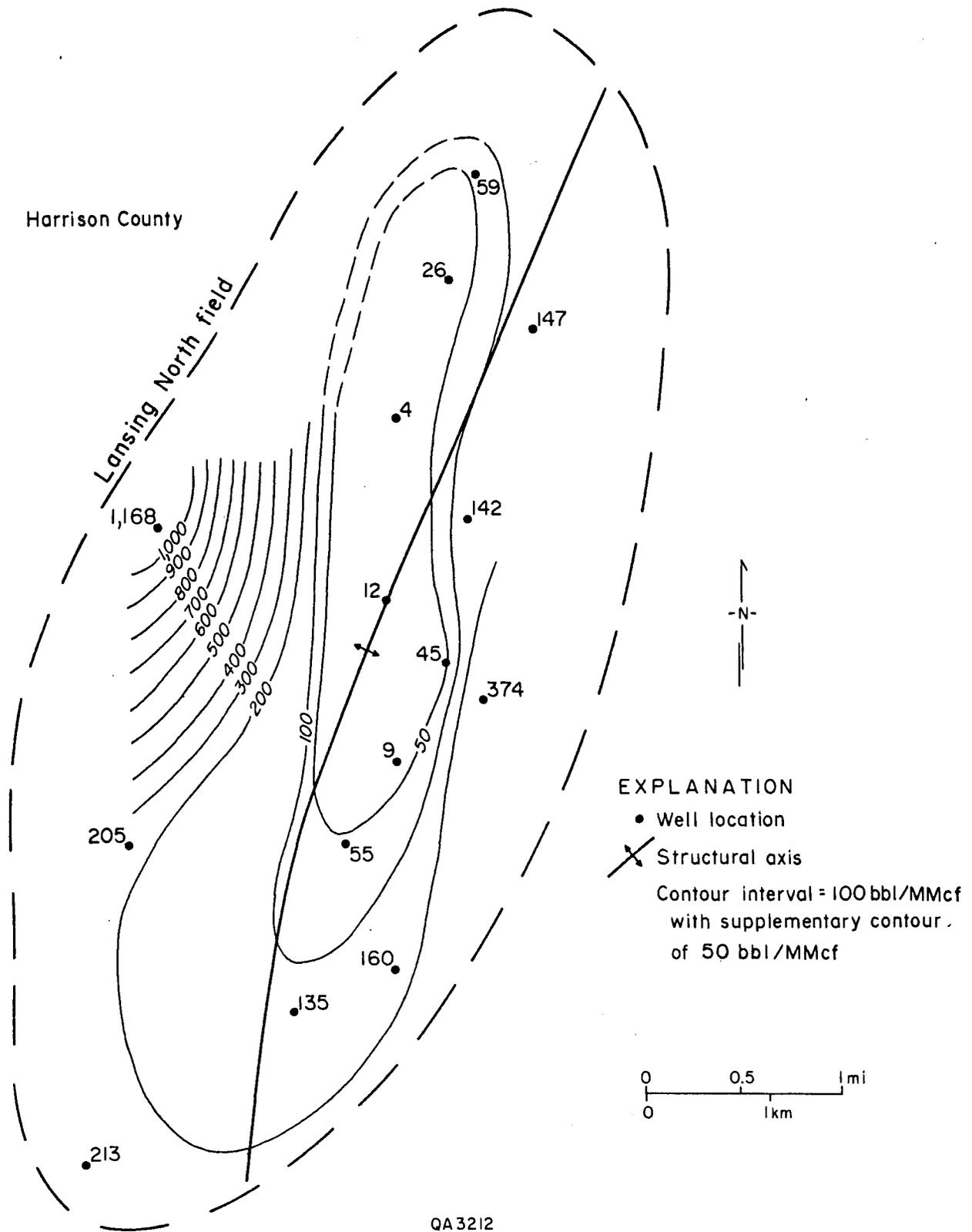
Figure 12. Distribution of initial water/gas production ratio in the Travis Peak Formation in Lansing North field.
