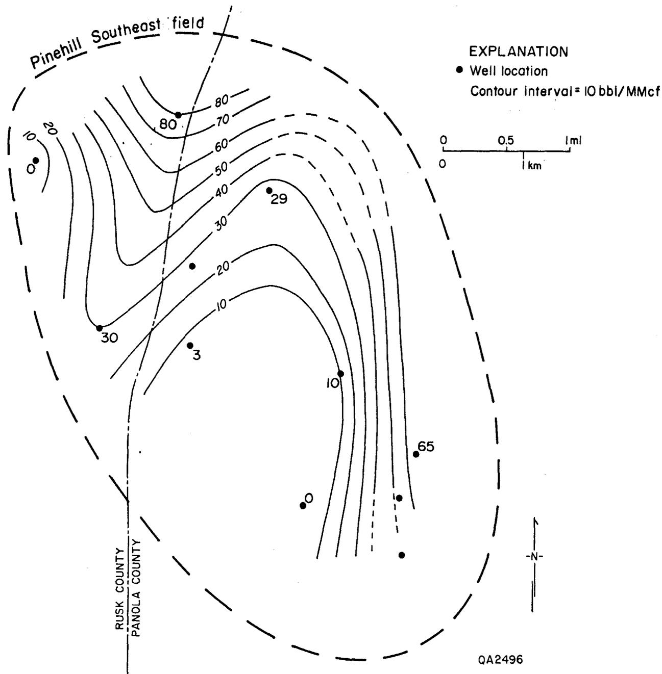
Figure 20. Distribution of initial water/gas production ratio in the Travis Peak Formation in Pinehill Southeast field.
