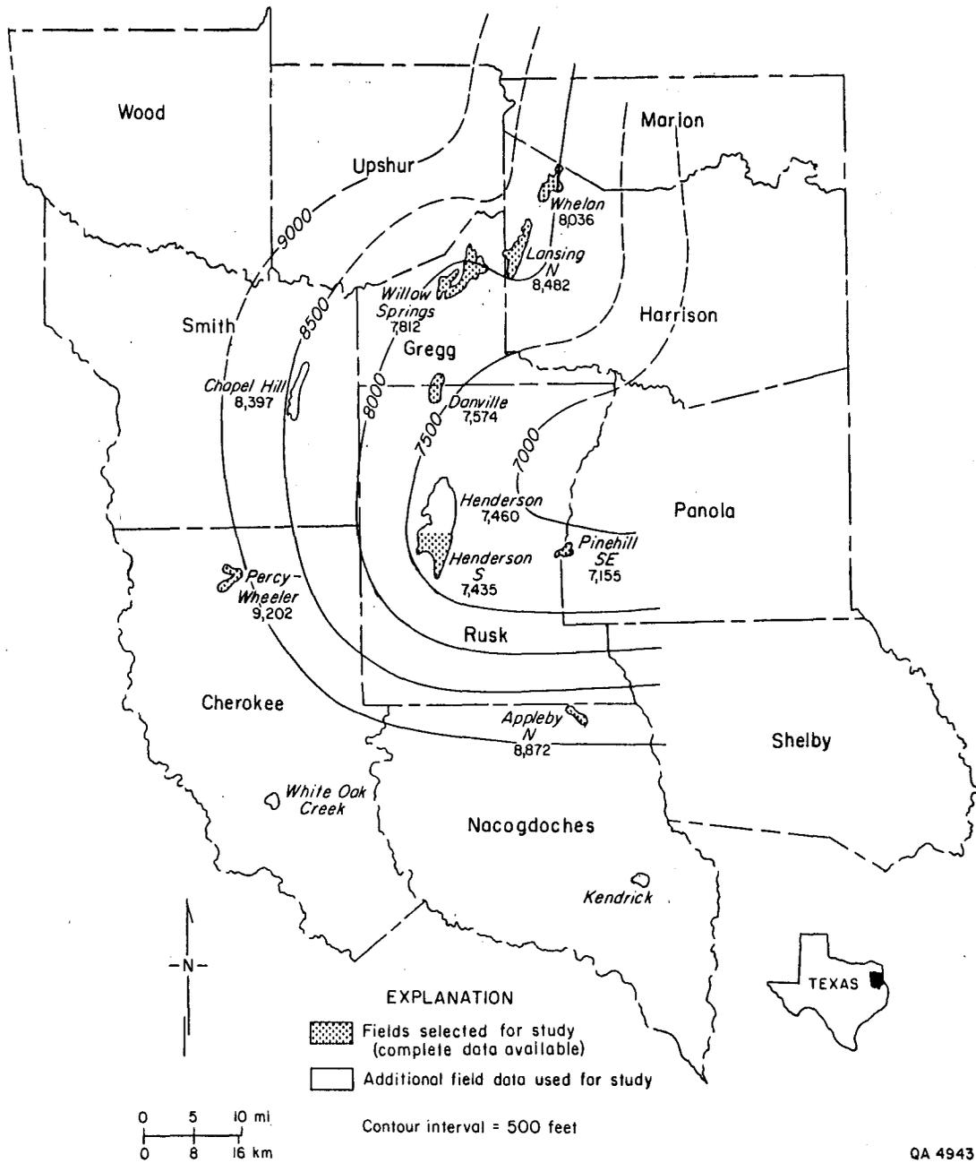
Figure 24. Distribution of field-average midpoint of perforated interval in the Travis Peak Formation, East Texas Basin.
