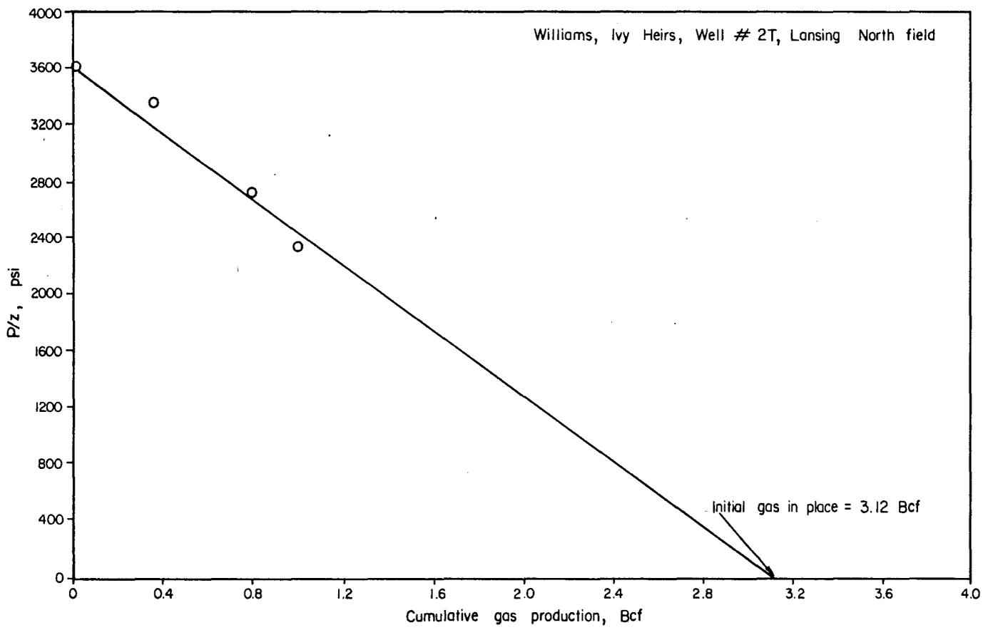
Figure 4. Plot of  $p/z$  versus cumulative gas production to estimate initial gas in place.
