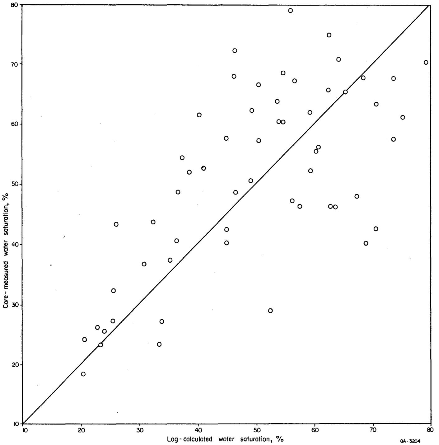
Figure 3. Comparison between core-measured water saturation and log-calculated water saturation for a well completed in the Travis Peak Formation, East Texas Basin.
