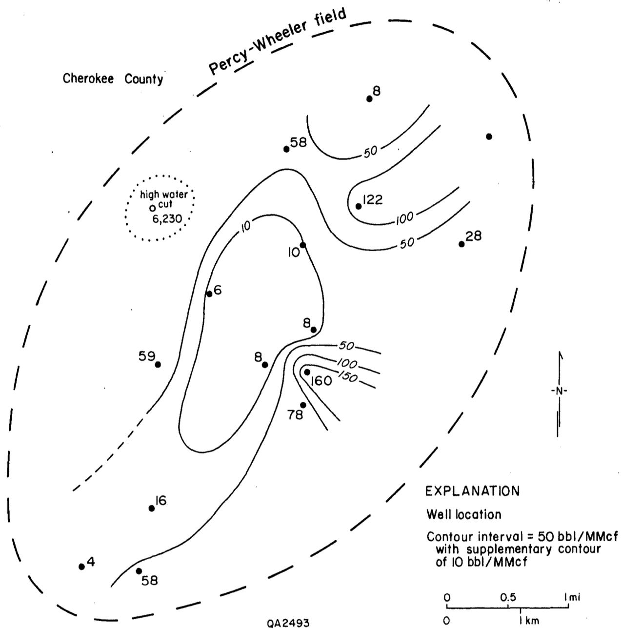
Figure 18. Distribution of initial water/gas production ratio in the Travis Peak Formation in Percy Wheeler field.
