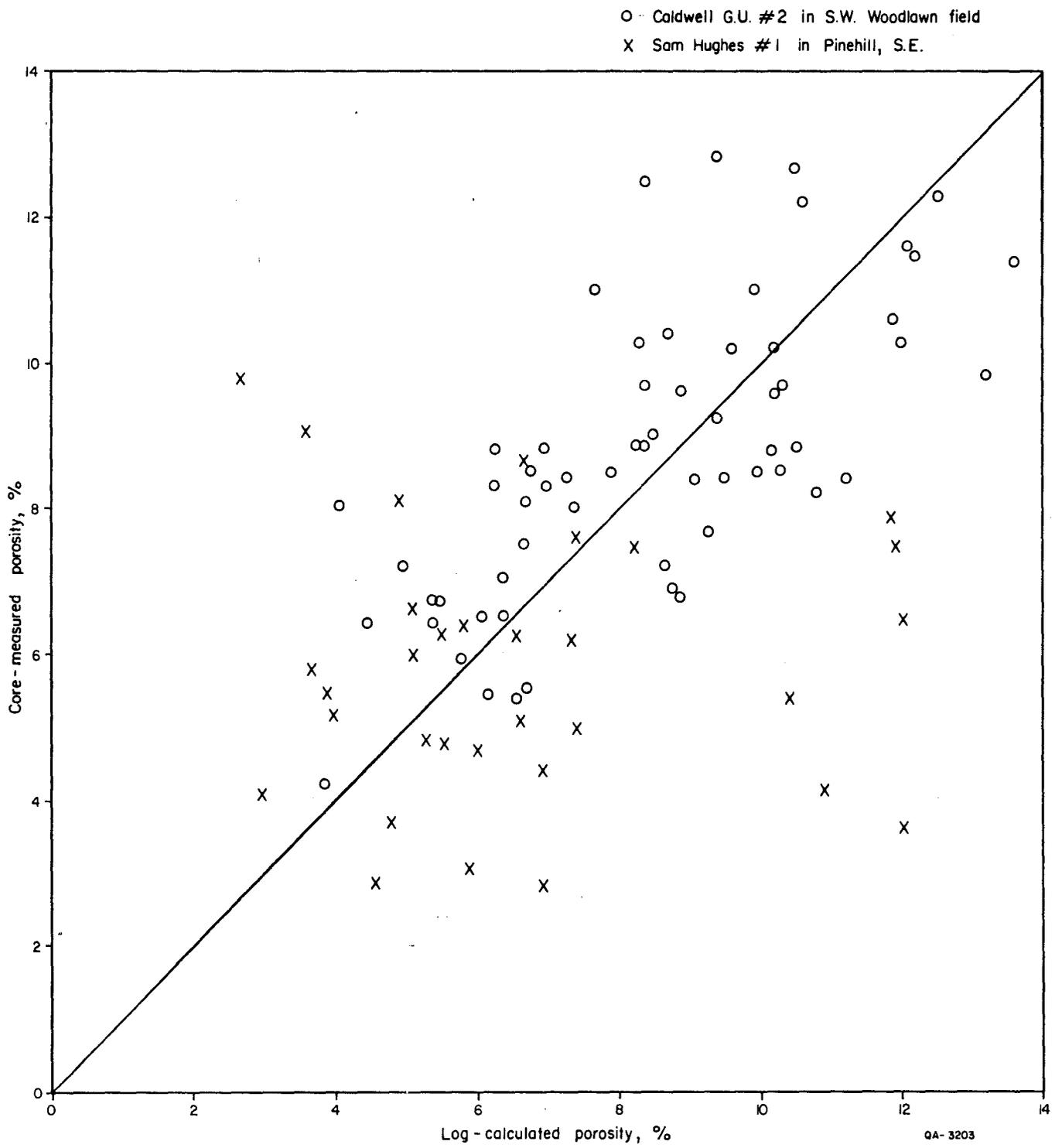
**Figure 2. Comparison between core-measured porosity and log-calculated porosity for the wells completed in the Travis Peak Formation, East Texas Basin.**
