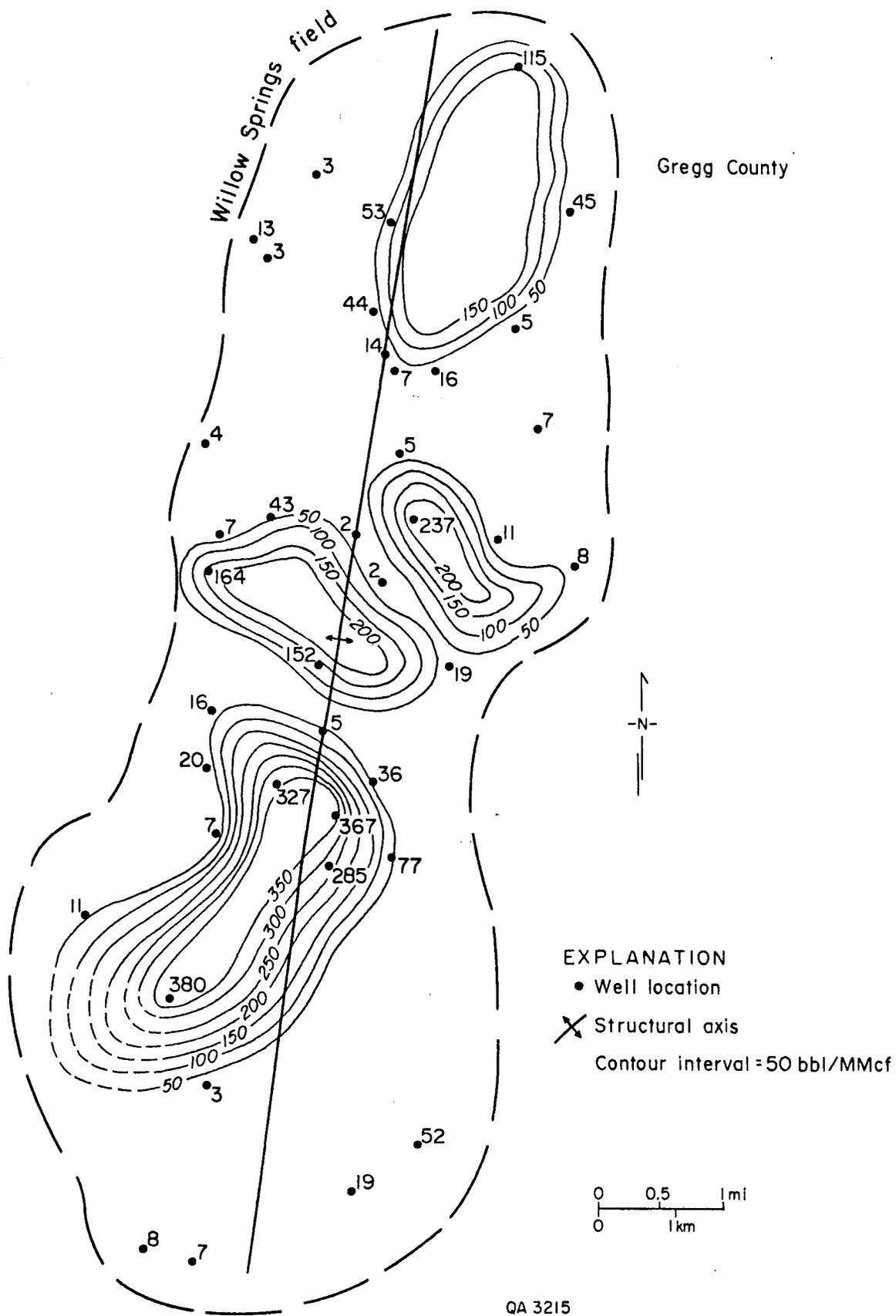
Figure 14. Distribution of initial water/gas production ratio in the Travis Peak Formation in Willow Springs field.
