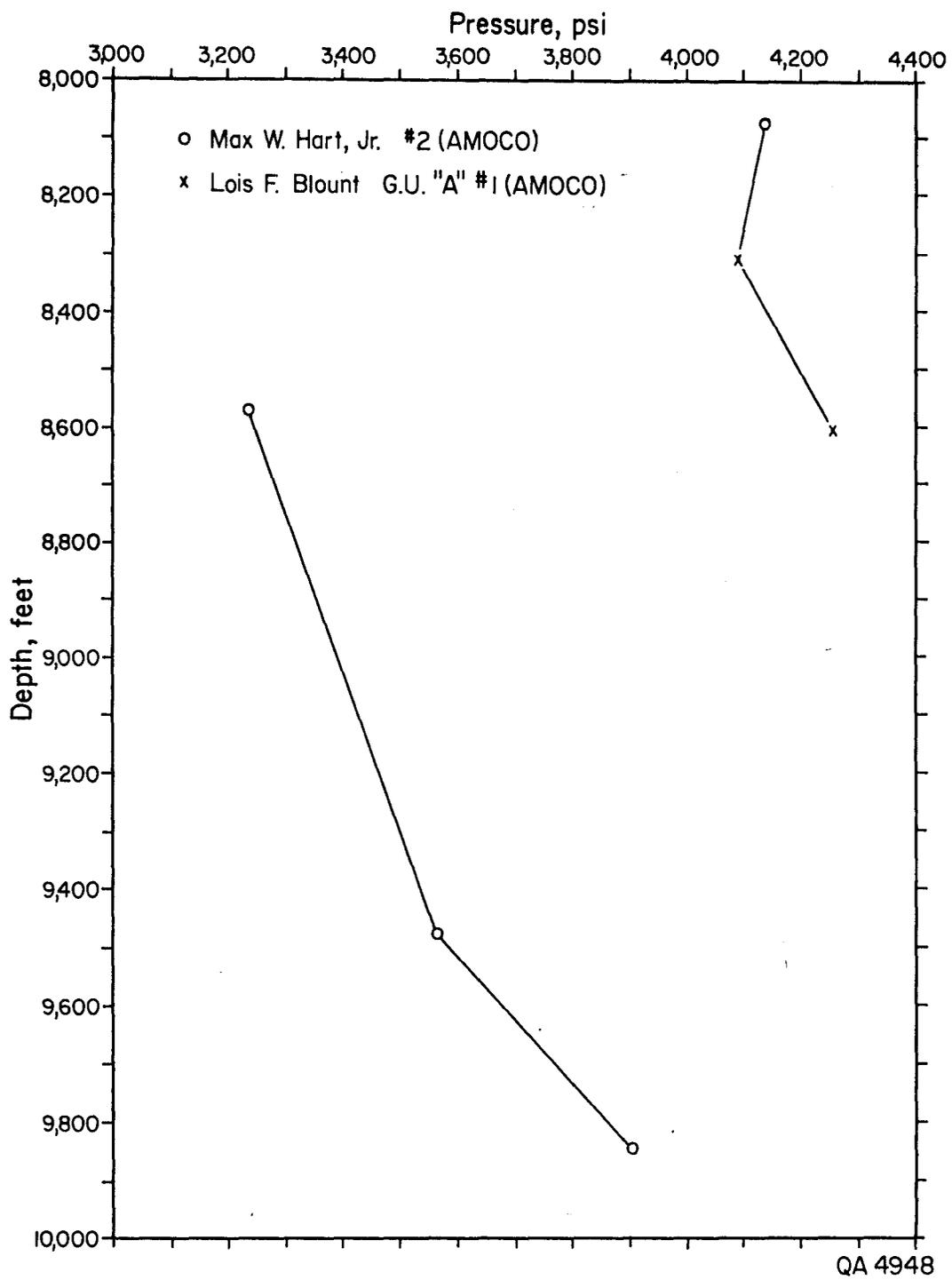
Figure 21. Pressure-depth plot for the data from two wells completed in the Travis Peak Formation in Appleby North field.
