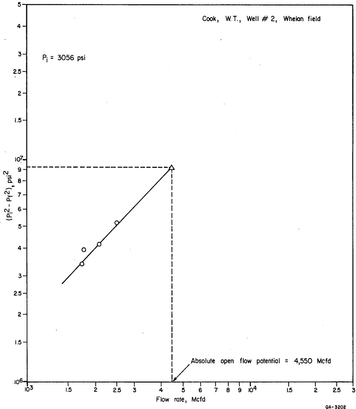
Figure 5. Plot of test flow rate versus pressure-square difference between reservoir and flowing wellbore pressure to estimate absolute open flow potential.
