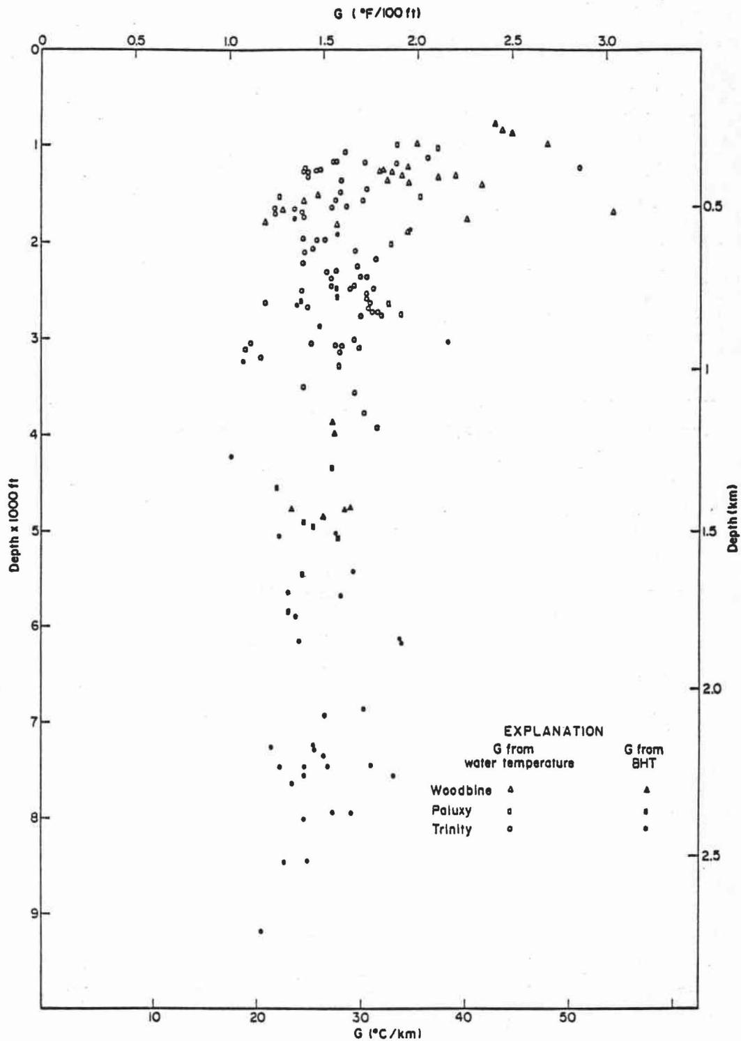
Figure 24. Geothermal gradient with respect to depth: Woodbine, Paluxy, and Hosston/Trinity aquifers, Dallas area.
