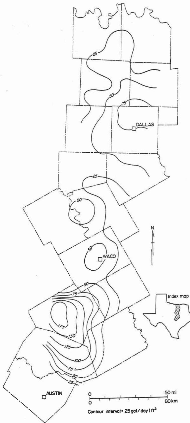
Figure 21. Moving average of hydraulic conductivity along part of the Balcones/Ouachita trend.
