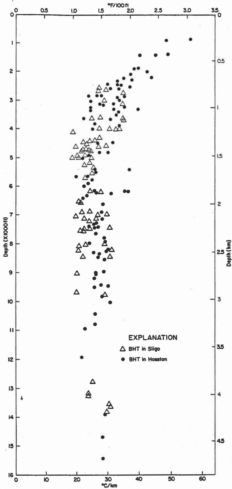
Figure 6. Geothermal gradient with respect to depth: Hosston and Sligo Formations.
