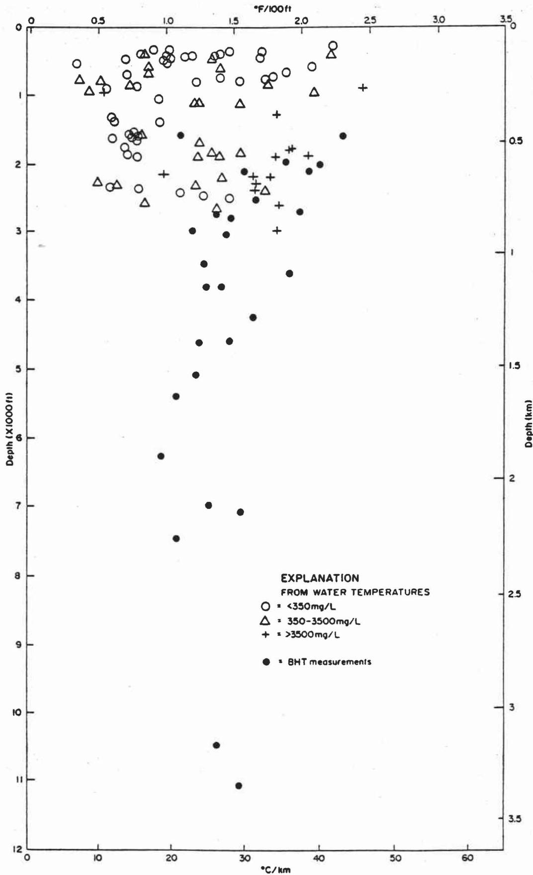
Figure 5. Geothermal gradient with respect to depth for Edwards Limestone; data derived from water temperatures and BHT measurements (from Woodruff, 1982).
