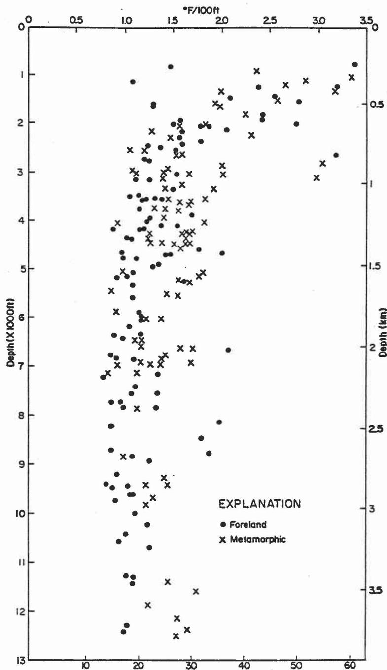
Figure 7. Geothermal gradient with respect to depth: Paleozoic Ouachita complex, Central Texas.
