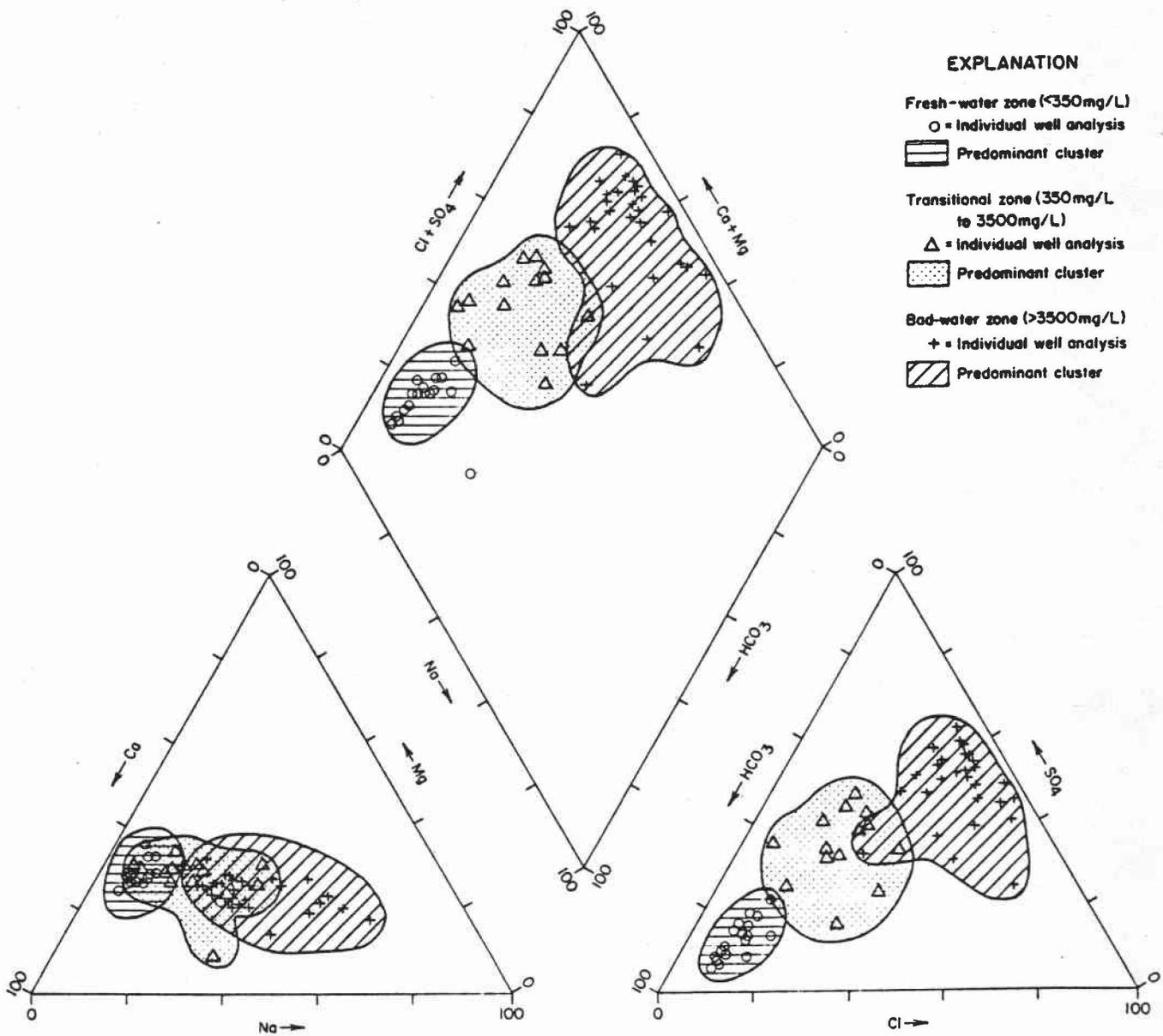
Figure 11. Piper diagram showing hydrochemical suites for ground water from the Edwards Limestone (from Woodruff, 1982).
