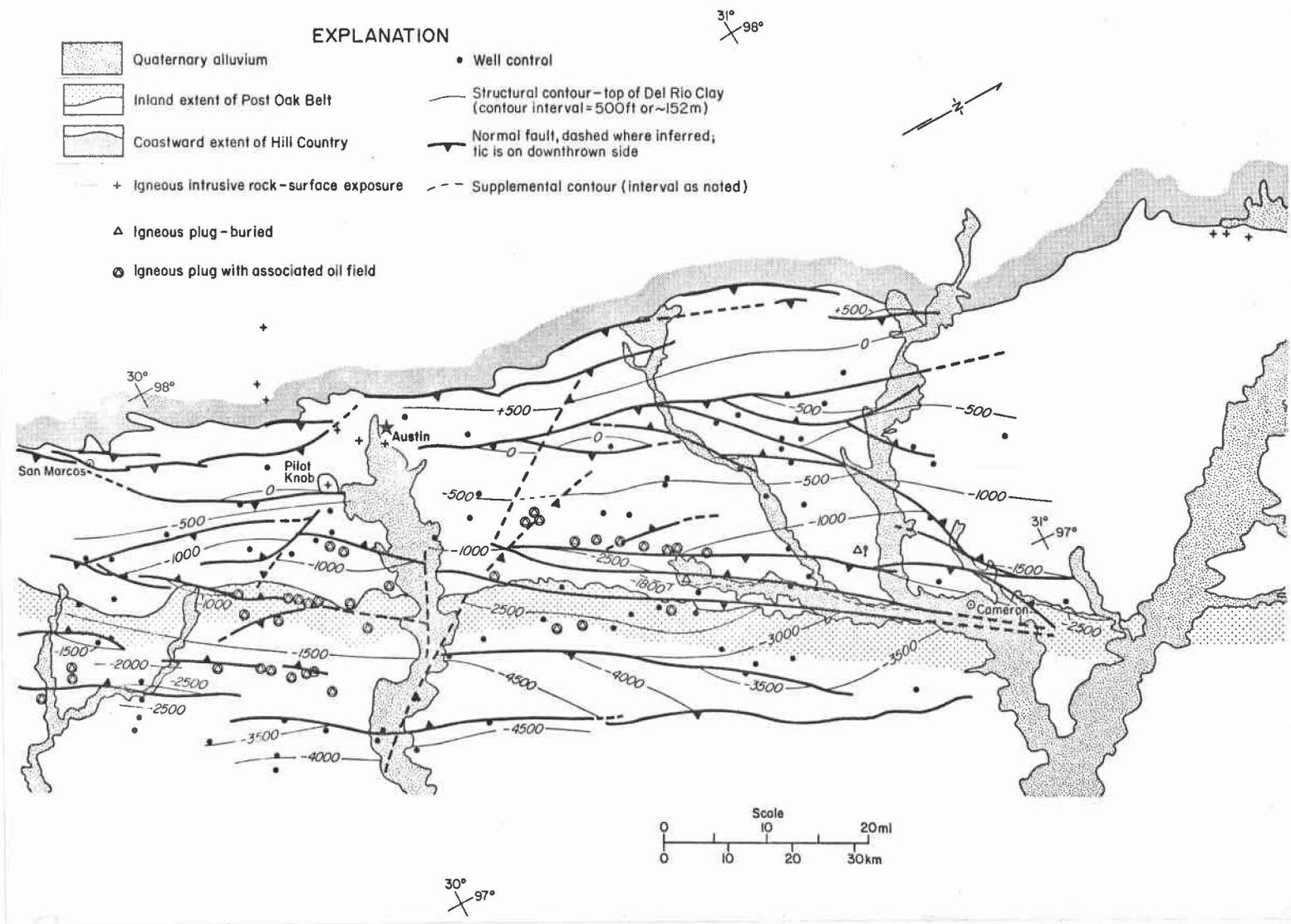
Figure 13. Subsurface structure, top of Del Rio Clay, Austin area.
