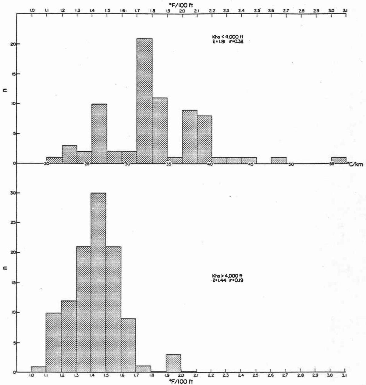
Figure 9. Histograms showing distributions of geothermal gradient values above and below the 4,000-ft (1.2-km) datum: Hosston Sand.
