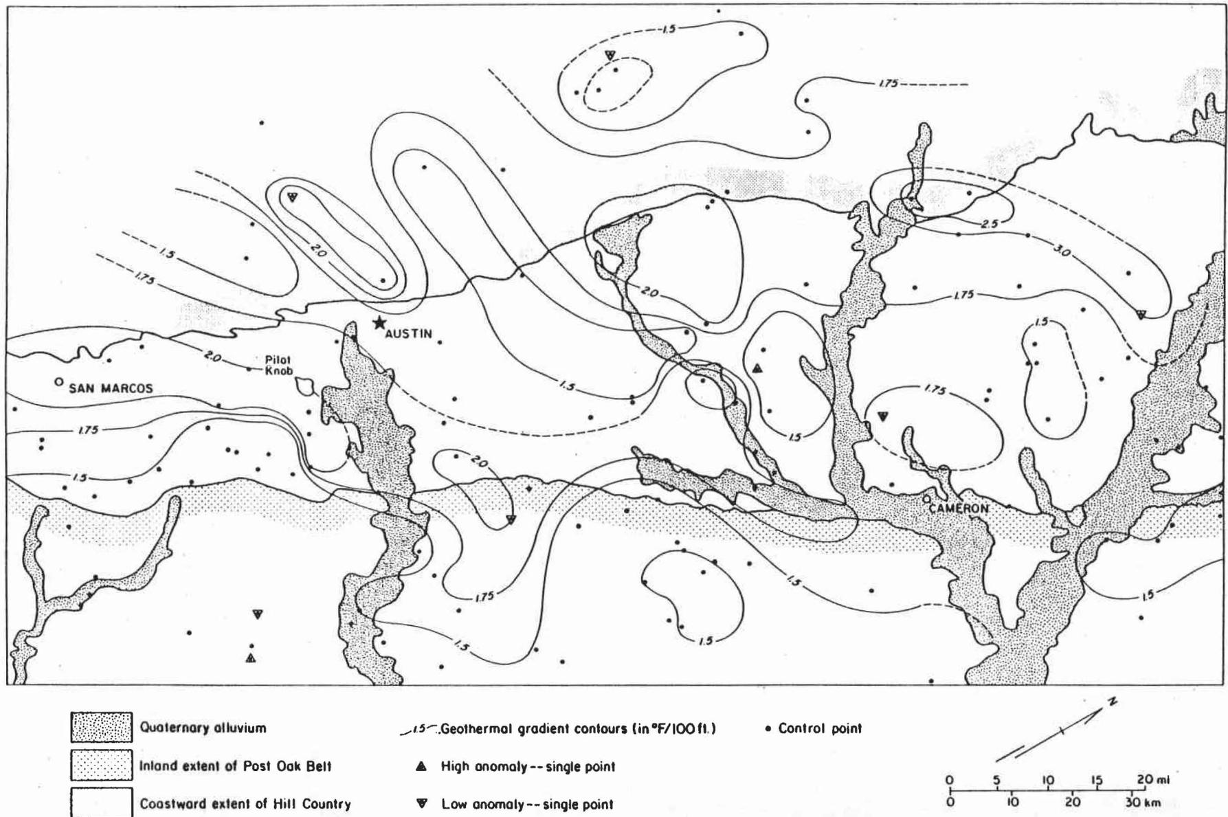
Figure 15. Composite geothermal gradient contours (that is, not discriminated according to specific horizon) Austin area (from Woodruff and Caran, 1981).
