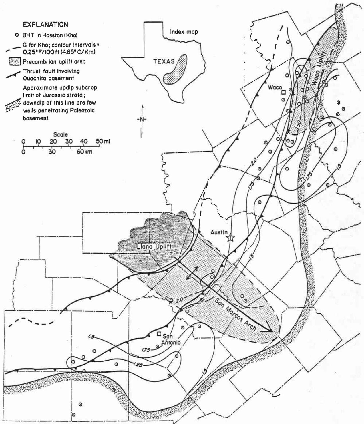
Figure 4. Geothermal gradient contours for Hosston/Trinity Sands.
