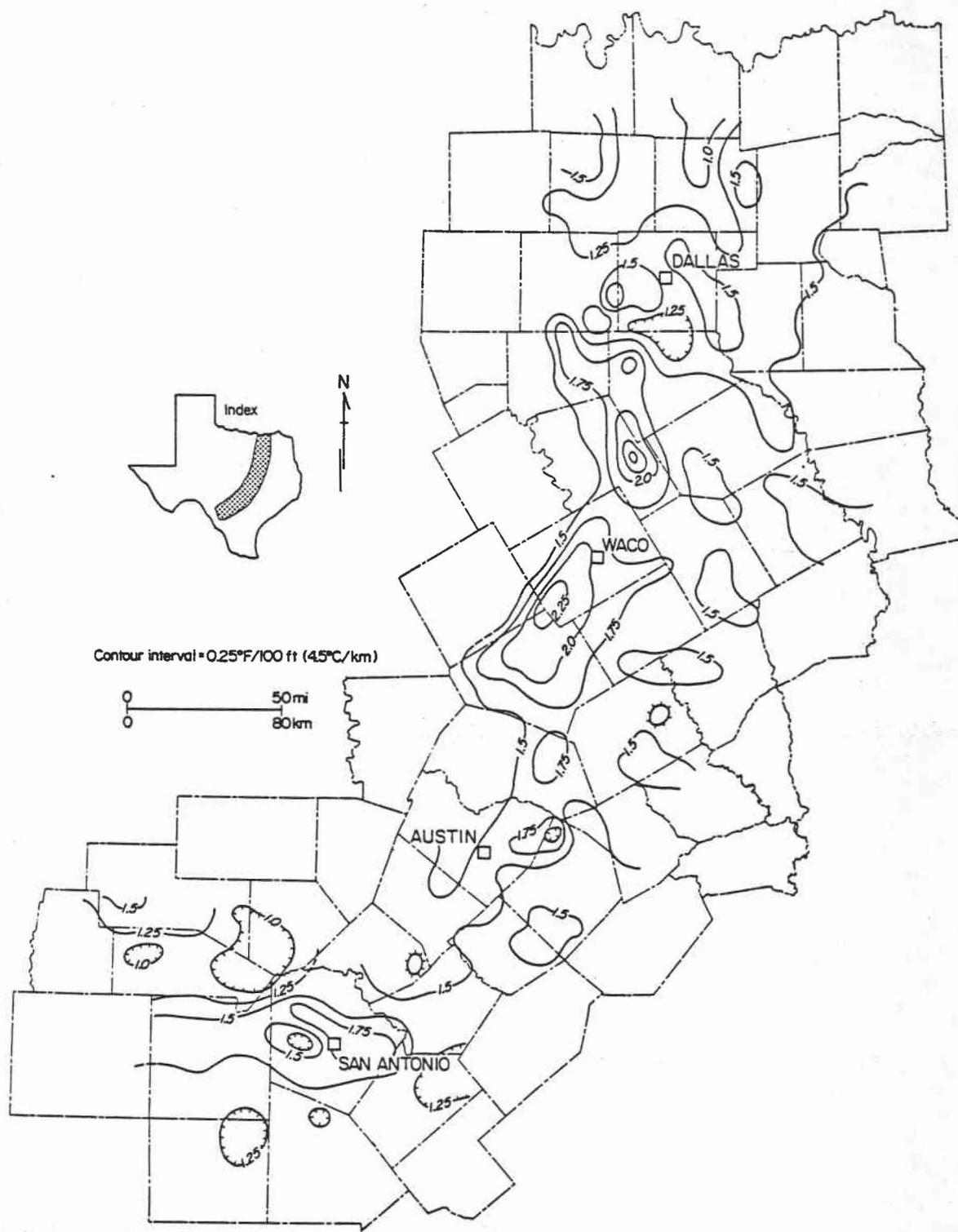
Figure 2. Moving average of geothermal gradients along part of the Balcones/Ouachita trend.
