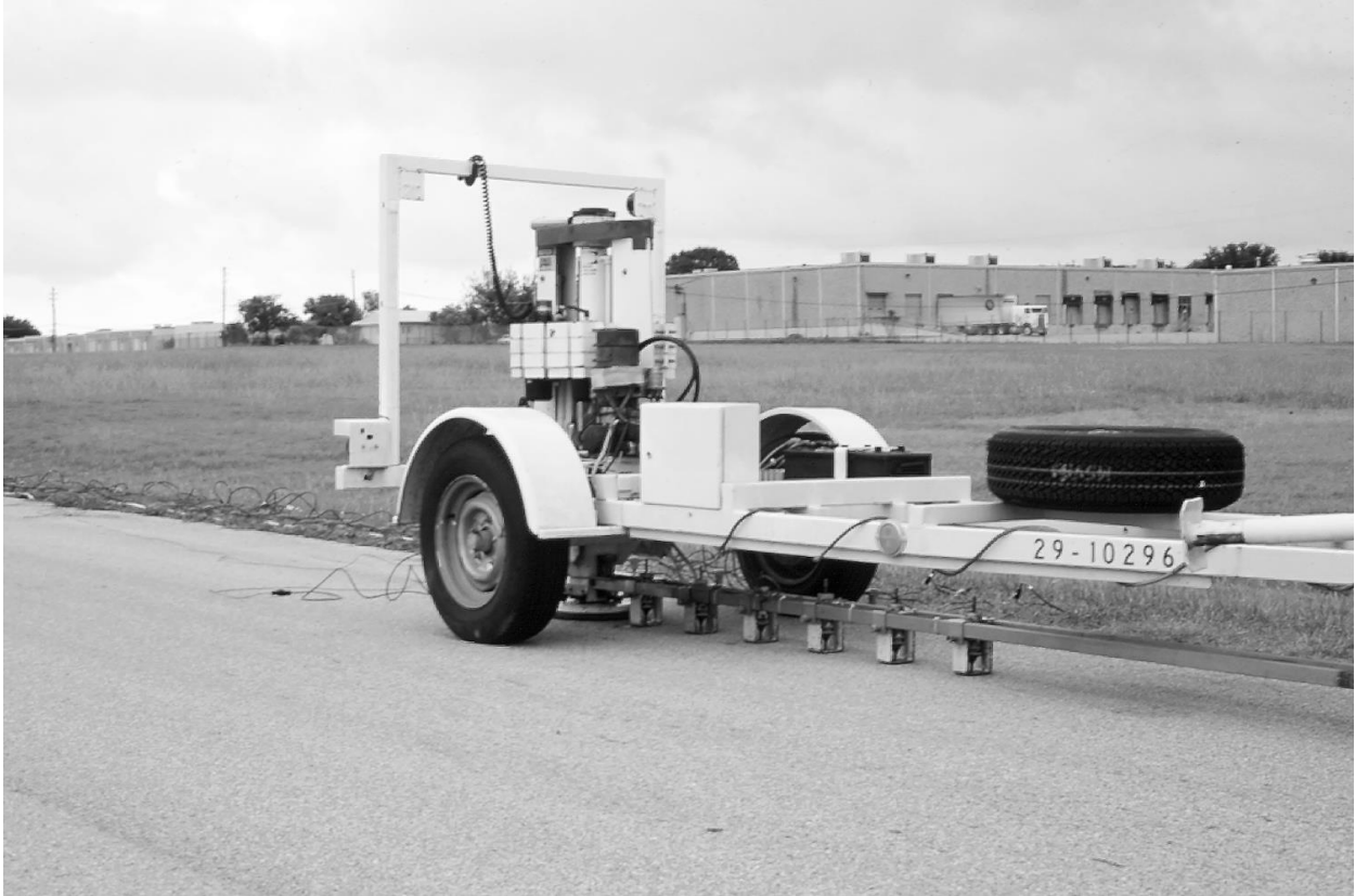
Figure 1. A Falling-Weight Deflectometer with detectors deployed on pavement.
