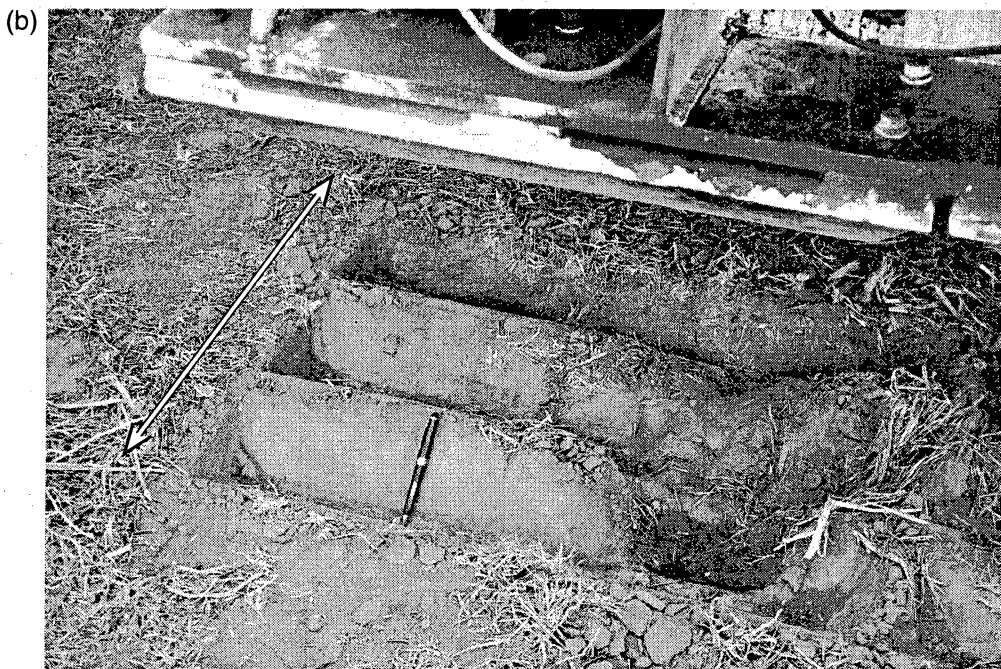
Fig. 2. (a) Minimal damage caused by a horizontal vibrator with a properly designed base cleat. The arrow shows the direction of pad motion. A writing pen is shown for scale. (b) Zoom view.
