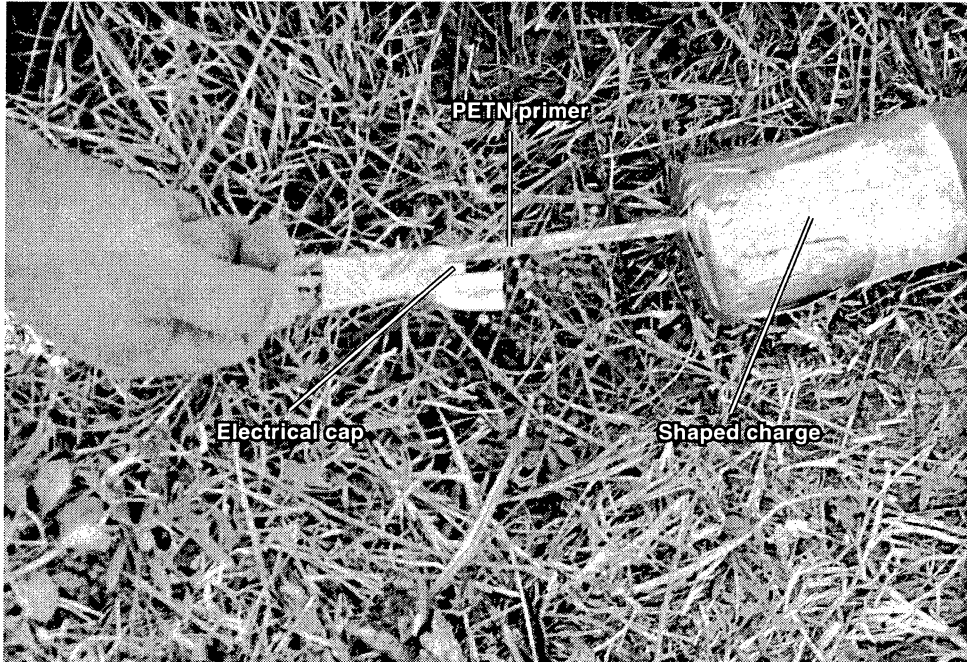
Fig. 11. (a) Low-velocity-emulsion shaped charge being prepared for detonation. (b) Proper union between cap and folded primer cord.
