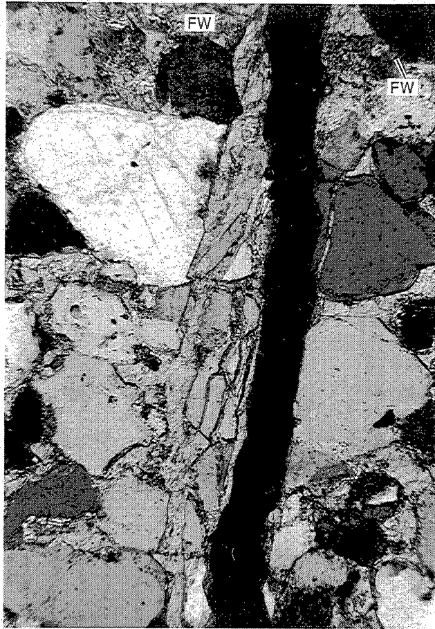
Figure 38. Calcite-filled fracture crosscutting grains and quartz cement, Enron Sawyer "A" 144 No. 5, depth 6,350 ft. Also note later handling-induced fracture (unfilled, dark). Bar = 1 mm. FW, fracture walls.
