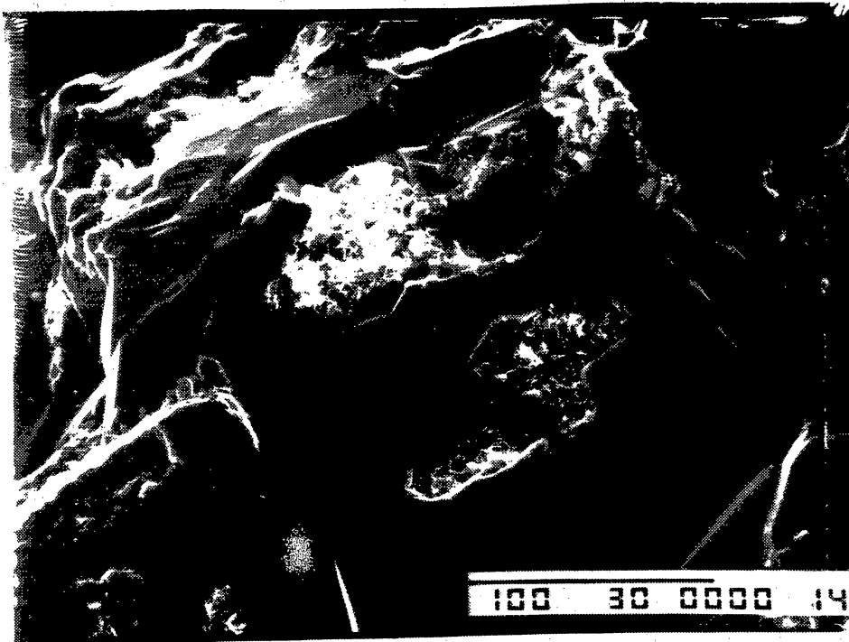
Figure 13. Quartz overgrowth engulfing illite and chlorite cement. Sample from a depth of 12,163.2 ft in the Wexpro Church Buttes No. 48 well. SEM photo by K. L. Herrington. Scale bar is 100 \mu\text{m} .
