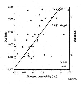
Figure 38. Plot of stressed permeability versus depth for 66 clean Travis Peak sandstones (from 10 md at 6,000 ft to 0.001 md at 10,000 ft).
