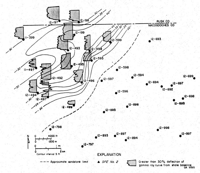
Figure 26. Net sandstone map for Sandstone X, lower Travis Peak, Zone 4, North Appleby field. Core, log, and map data indicate that this sandstone was deposited in a northeast/southwest-oriented channel belt. Gamma-ray log signatures are generally blocky to upward-fining.
