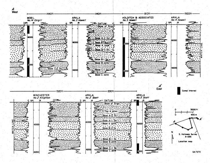
Figure 19. Cross section of upper Travis Peak producing sandstones in the area around the SFE No. 1 well.
