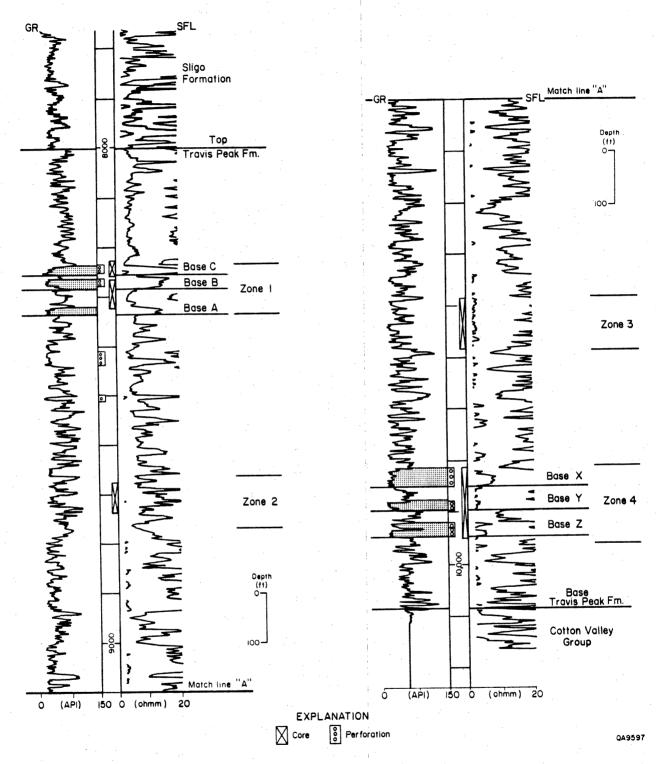
Figure 22. Gamma-ray and resistivity (SFL) logs and informal nomenclature for the Travis Peak Formation in SFE No. 2. Cored and perforated intervals are shown.
