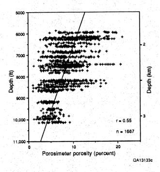
Figure 34. Plot of porosimeter porosity versus depth for 1,687 Travis Peak sandstone samples. Both the mean and range of porosity values decrease with depth.
