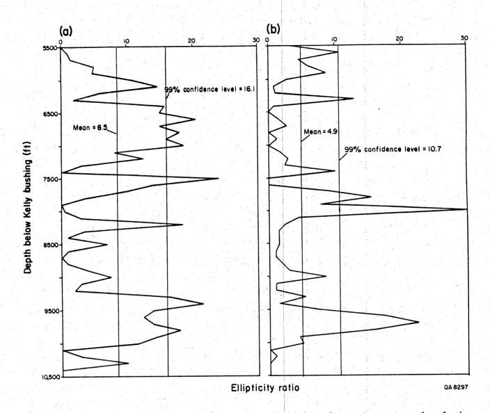
Figure 60. Plots of ellipticity ratio vs. depth below Kelly bushing (approximate ground surface). (a) Northeast peaks. (b) Northwest peaks. No clear distinction exists between the northeast and northwest peaks relative to depth below Kelly bushing.
