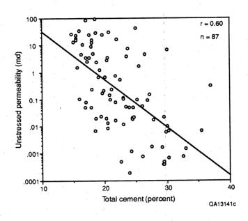
Figure 42. Inverse relationship between total cement volume and unstressed permeability in clean sandstones. Volume of authigenic cement is a major control on permeability in Travis Peak sandstone.
