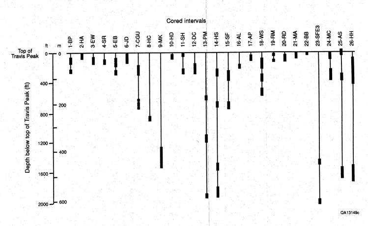
Figure 7. Cored intervals plotted by depth below the top of the Travis Peak. See table 1 for explanation of abbreviations.
