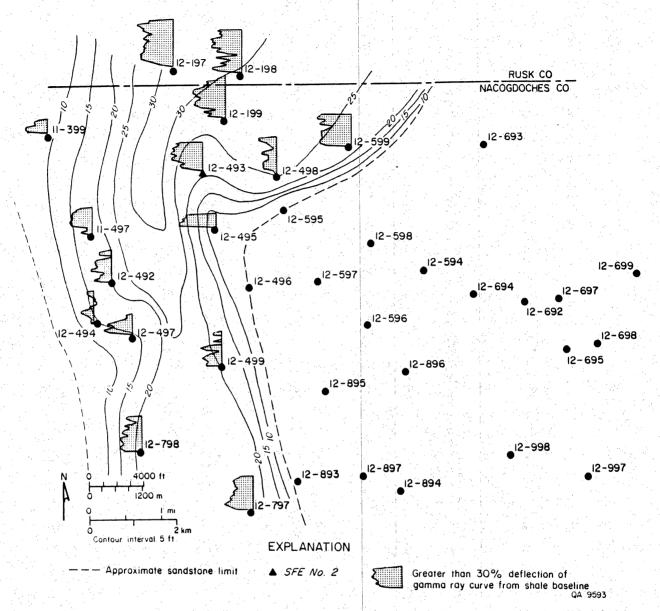
Figure 25. Net-sandstone map for Sandstone B, upper Travis Peak Zone 1, North Appleby field. Core, log, and map data indicate that this sandstone was deposited in a north/south oriented channel belt. Gamma-ray log signatures are generally blocky to upward-fining.
