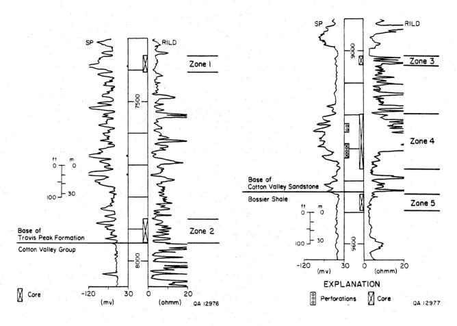
Figure 27. Gamma-ray and resistivity logs of lower Travis Peak Formation, lower Cotton Valley Sandstone, and Bossier Shale, SFE No. 3 well, showing cored and perforated intervals.
