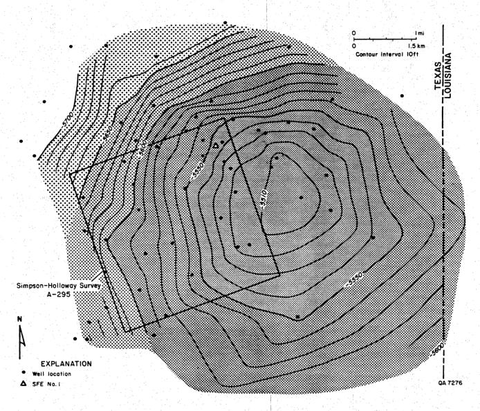
Figure 16. Structure map of the top of the lowest carbonate bench in the Sligo Formation, Waskom field, Harrison County, Texas. Location of SFE No. 1 (Holditch & Associates Howell No. 5) is shown.
