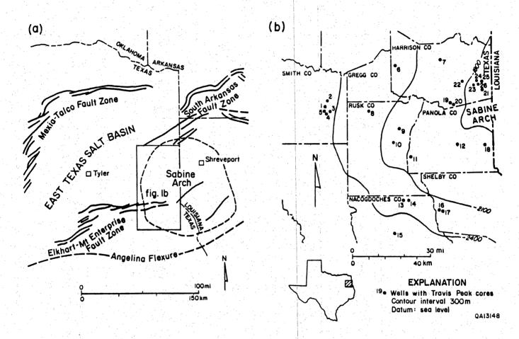
Figure 1. Location of study area and wells. (a) Structural setting of the Travis Peak Formation, East Texas. (b) Location of wells for which Travis Peak cores are available and structure on the top of the Travis Peak. See table 1 for well names.
