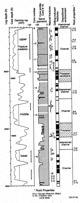
Figure 46. Core gamma ray log, core profile, fracture distribution, and environmental interpretation for core 9-15, Holditch SFE No. 2 well. Static rock property measurements from core plugs in this interval are also indicated. This core interval illustrates numerous fractures in lower Travis Peak Formation.
