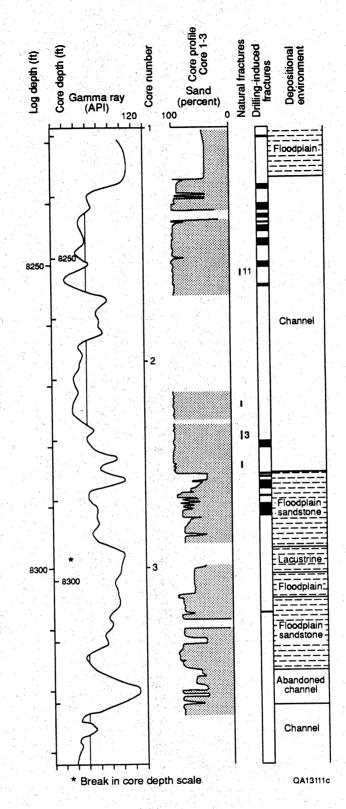
Figure 45. Core gamma ray log, core profile, fracture distribution, and environmental interpretation for core 1-3, Holditch SFE No. 2 well. Note that few natural fractures occur in this interval.
