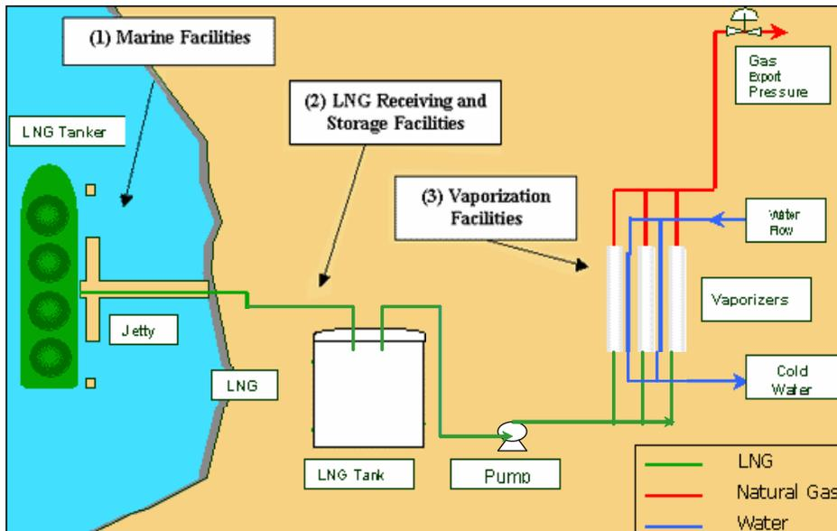
Source: BP LNG. Note that type of vaporization process and related water requirements may vary. See Appendix 1: Descriptions of LNG Facilities for details.
