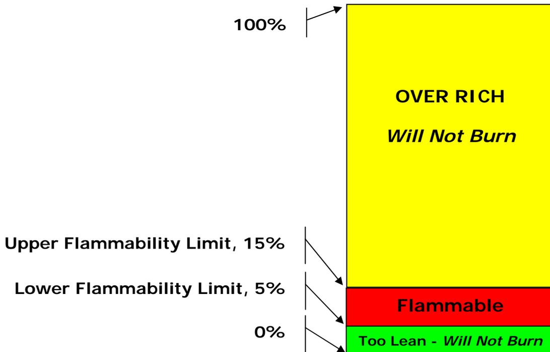
A comparison of the properties of LNG to those of other liquid fuels, as shown in Table 1 below, also indicates that the Lower Flammability Limit of LNG is generally higher than other fuels. That is, more LNG vapors would be needed (in a given area) to ignite as compared to LPG or gasoline.
