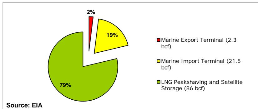
Despite the relatively low percentage of total gas storage capacity represented, the high daily deliverability of LNG facilities makes them an important source of fuel during winter cold snaps. LNG facilities can deliver up to about 11 BCFD (BCF per day), or the equivalent of 14 percent of the quantity of gas supply that can be delivered from underground storage locations in the U.S.
