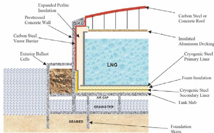
LNG storage tanks are fitted with thermal insulation to prevent heat transfer into the cargo tank, to reduce boil-off of the LNG, and also to protect the structure from cryogenic temperatures that would cause brittle fracture. The insulation is either "sandwiched" between the inner hull and primary
