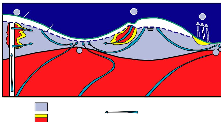
Figure 1. Conceptual model of salinity sources. Potential sources are (1) natural discharge of brine through permeable stratigraphic units, fractures and joints; (2) upward flow of brine through inadequately plugged and leaky boreholes; (3) infiltration of saline water beneath brine disposal pits; and (4) evaporative concentration of shallow groundwater.
