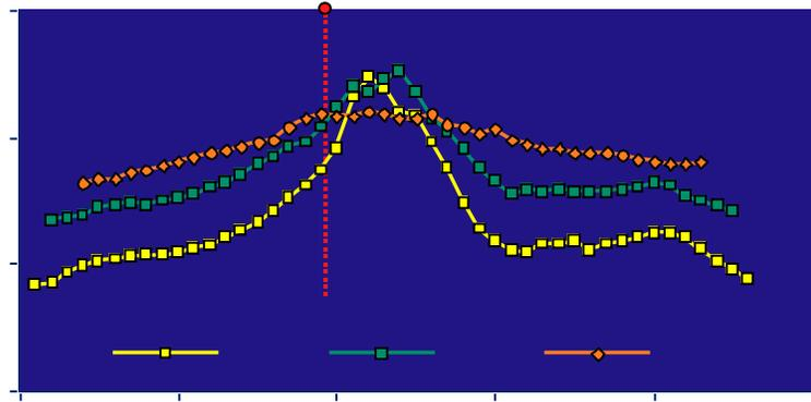
**Figure 5.** Apparent ground conductivity profile across site 76 measured using a ground-based induction instrument at 10-, 20-, and 40-m coil separations. Wider coil spacings correspond to deeper exploration depths. The line crosses the abandoned Vancil 1 well where a highly conductive zone is apparent at all exploration depths, is centered a few meters from the well, and broadens with depth.
