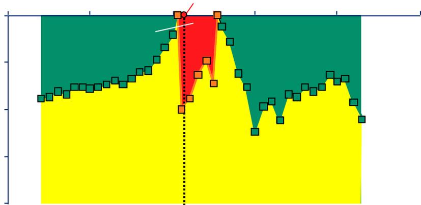
**Figure 6.** Two-layer conductivity model that fits ground-based electromagnetic data collected at site 76. Vancil 1 is flanked by highly conductive ground that represents a zone of saltwater infiltration. Although this well shows no evidence of brine leakage at the surface, on the basis of airborne and ground-based geophysical data, we interpret it to be leaking brine.
