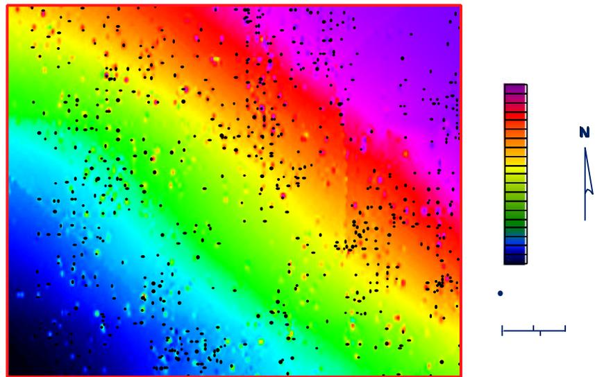
**Figure 2.** Map of total magnetic field strength. Superimposed on the southwest-northeast regional gradient are small anomalies that correlate well with known oil and gas well locations (black circles). Well locations provided by the Texas Railroad Commission.
