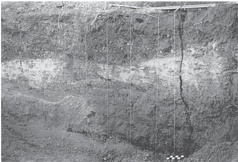
Fig. 2 Location of fracture and five sampling profiles parallel to fracture beneath ponded surface. The strata are of fine-grained material at the ponded surface, underlain by gravel, a petrocalcic layer (light-colored), fine sediment, and gravel at the base.
