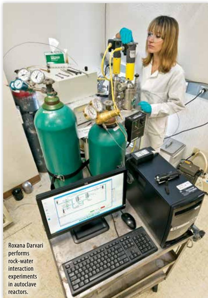
Roxana Darvari performs rock-water interaction experiments in autoclave reactors.
