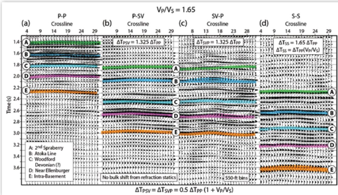
Four seismic images extracted from wave fields produced by a vertical-vibrator source. Two images (P-P and P-SV) are produced by the direct-P mode, and two images (SV-P and S-S) are produced by the direct-SV mode. A, B, C, and D are depth-equivalent horizons in the four image spaces. Data collected in the Midland Basin.
