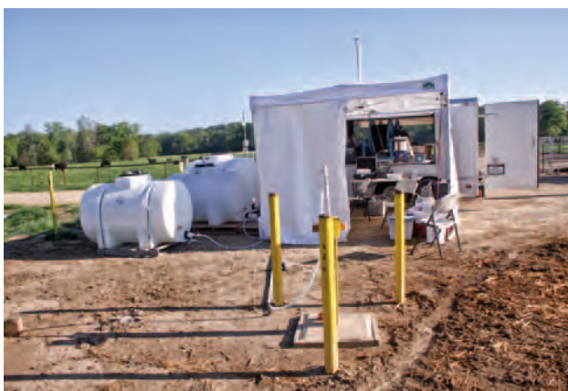
Push-pull test conducted at Cranfield site for assessing potential impacts of CO 2 leakage from geological CO 2 sequestration on groundwater drinking resources.
