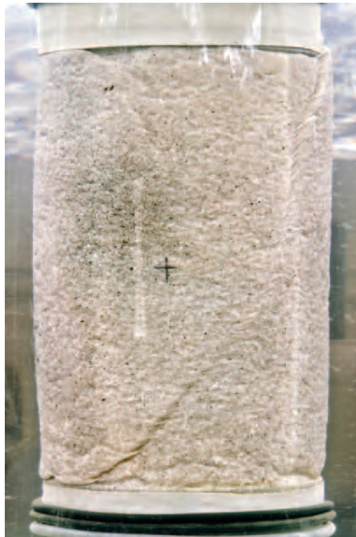
A natural sand specimen developing a failure plane (shear band) during a triaxial test.
