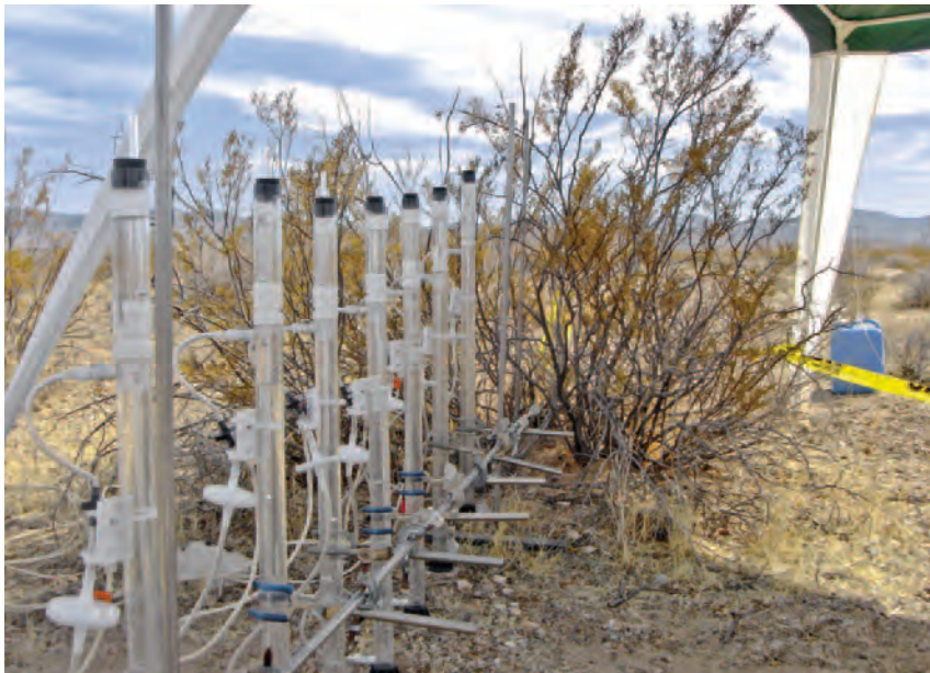
Fine-scale measurements of infiltration capacity around a shrub in the Mojave Desert.
