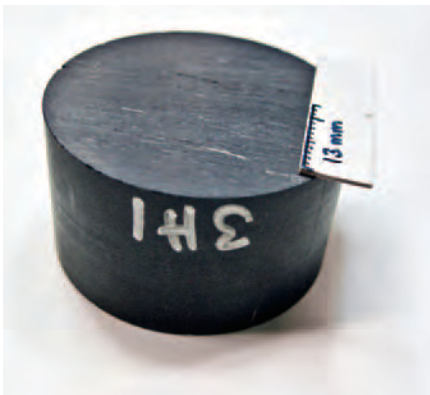
Barnett shale core plug used for gas-permeability measurement.
