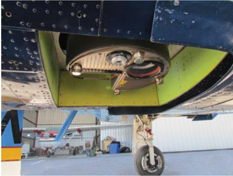
Sensor window of the Optech Titan multispectral lidar.
