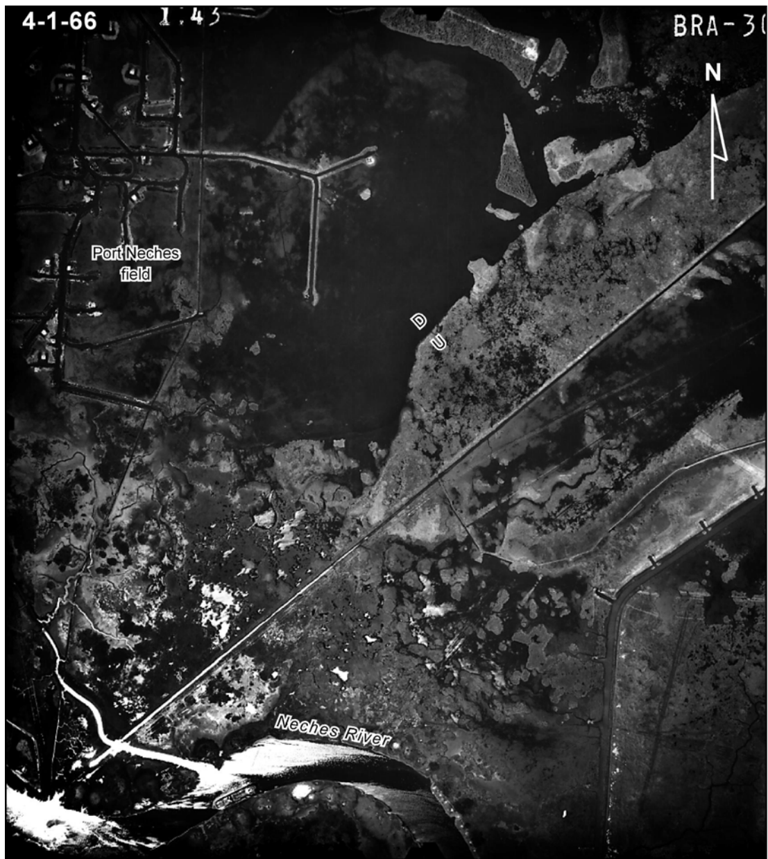
Figure VI. Fault in Neches River valley downthrown toward the oil and gas field. Dark areas of open water increase on the downthrown side (D) of the fault relative to the upthrown side (U). This photograph was taken by the U.S. Department of Agriculture in 1966. The fault could not be seen on photographs taken in 1956. From White and Morton (1997).
