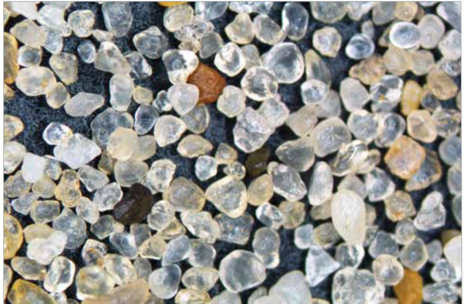
Rounded, relatively uniform grains like these from the Kermit sand are desirable for applications like fracking.
