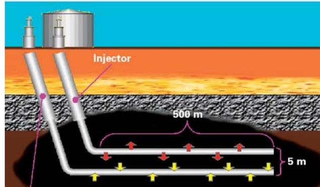
Another technique that is used is that of the injection of diluent into the reservoir to reduce viscosity. One process involves the injection of diluent vapors in order to heat the heavy oil and also reduce its viscosity via the incorporation of the solvent into the heavy oil matrix. One such technique is commonly called VAPEX. VAPEX has shown interesting results in laboratory and core experiments but has not been tested at the commercial scale.
