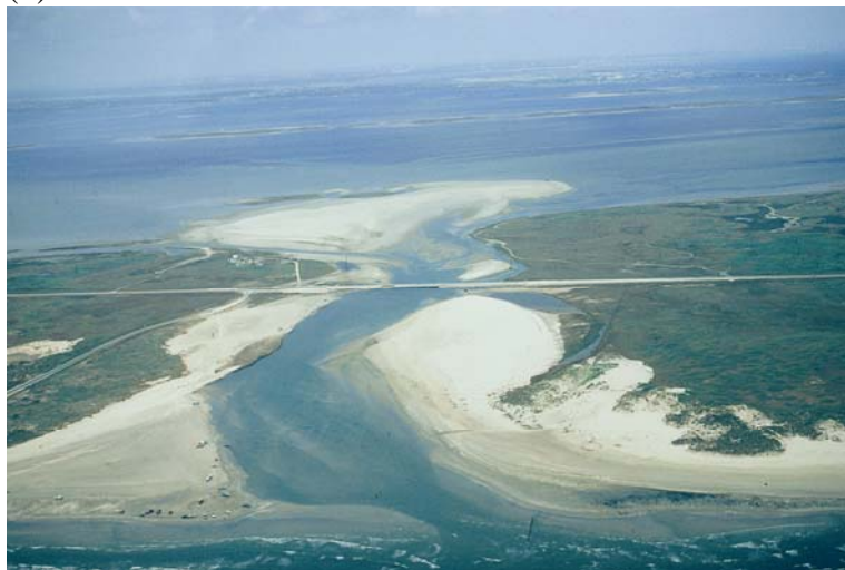
Figure 6. Vertical aerial photograph (2002) of Corpus Christi Pass, a hurricane washover channel located at the southern end of Mustang Island (a), and Corpus Christi Pass a few days after Hurricane Allen made landfall in August of 1980 (b). Longshore currents and sand migration along the Gulf shoreline (foreground) close the pass between hurricanes, and the barren sand and washover fan deposits become vegetated with salt tolerant plants.
