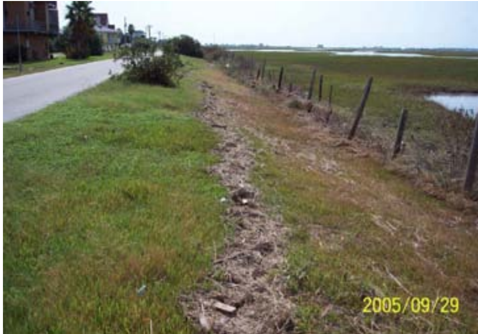
Figure 33. Grass debris line left by Hurricane Rita at 0.6 to 1-m above mean sea level. Jamaica Beach on West Bay side of Galveston Island.
